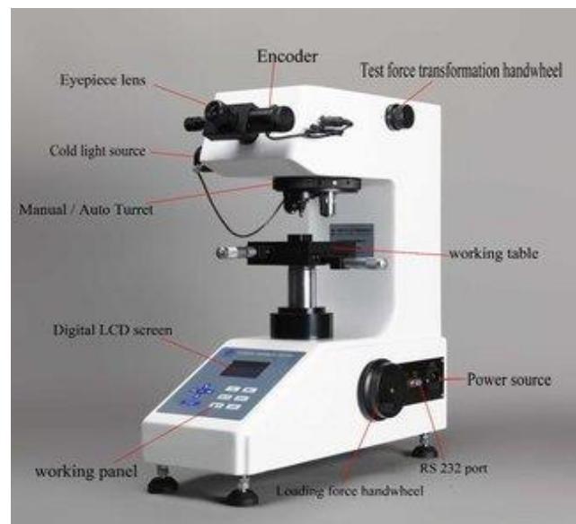
Figure 2: Vickers hardness testing machine components [7]
