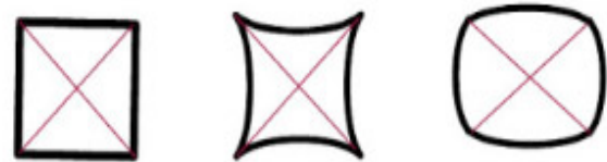
Figure 1: Form of penetration traces [7]
