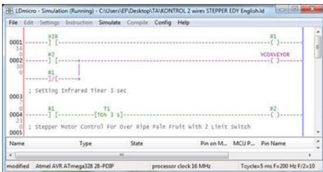
Figure 6.b: Conveyor Mode Simulation moves after Infrared is inactive for 3 seconds.
