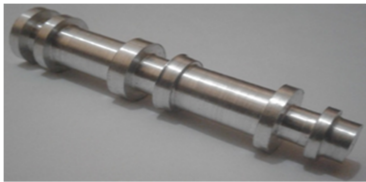
Figure 5: Result of the master cylinder piston used NC lathe machine for parallel to surface scheme
