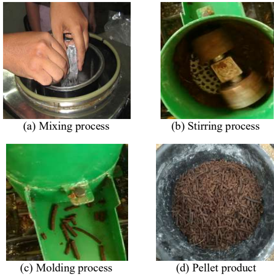
Figure 1: The process of prepared materials of biomass pellet
