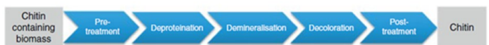
Figure 3. Steps in the process of isolation and purification of chitin from biomass adapted from Bastiaens et al., 2019
