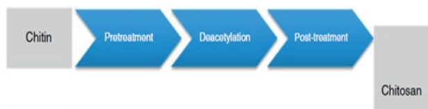
Figure 4. Stages in the process of converting chitin into chitosan adapted from Bastiaens et al. , 2019
