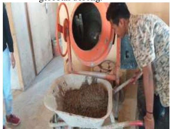
**Gambar 4.7** Pengambilan sample uji slump
