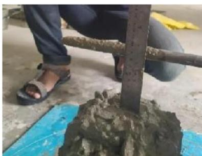
**Gambar 1.** Slump Test Campuran Beton
