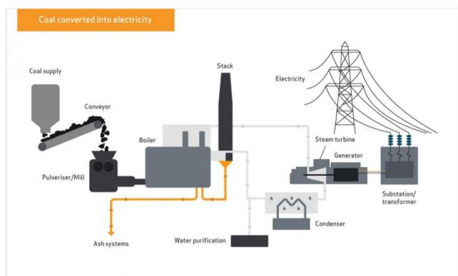
**Figure 1** The pulverized coal combustion (PCC) system uses to convert coal to electricity. Adapted from World Coal Association. Copyright 2013 by VGB Power Tech.
