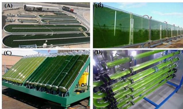
**Figure 5** The Algae cultivation methods. A) Natural, B) Artificial (flat plate photobioreactor), C) Tubular photobioreactor and D) Column photobioreactor (Adeniya et al., 2018)
