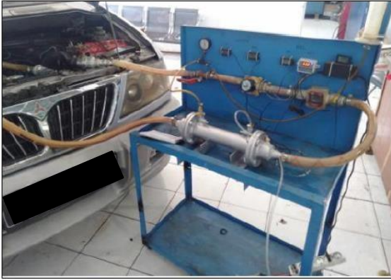
Gambar 7. Mesin Diesel dan Sistem Heat Exchanger
