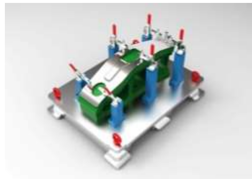
Gambar 5. CF (checking fixtures) Sumber: (Grabcad, 2021)
