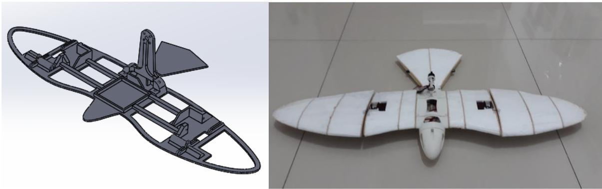
**Gambar 2. Kiri: platform simulasi, kanan: airframe UAV meniru burung.**
