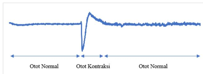
Gambar 2. Sinyal Electromyogram(EMG).
