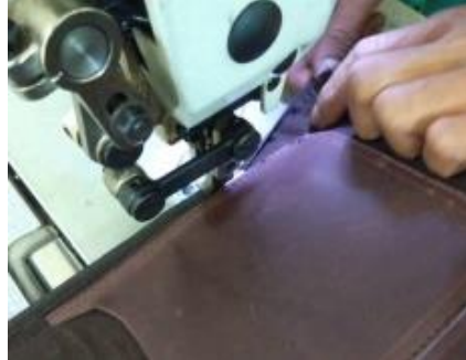
Figure 29. Installing the side cover of the bag (Photo: Mutiana Pramita Sari, 2020)
