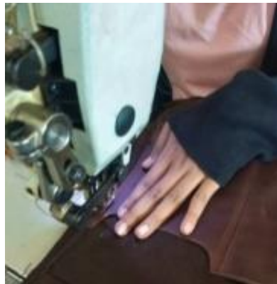
Figure 27. Inner pocket installation process (Photo: Mutiana Pramita Sari, 2020)
