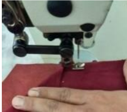
Figure 26. Furing installation process (Photo: Mutiana Pramita Sari, 2020)
