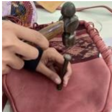
Figure 31. Installing the snap button (Photo: Mutiana Pramita Sari, 2020)
