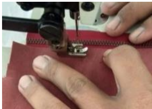
Figure 30. Installing the zipper (Photo: Mutiana Pramita Sari, 2020)
