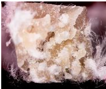
Figure 9. Macroscopic view of specimen fracture at volume fraction of 7.5% cotton fiber
