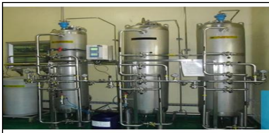
Figure 10. Softener Filter (Source: PT. Nulab Pharmaceutical Indonesia)
