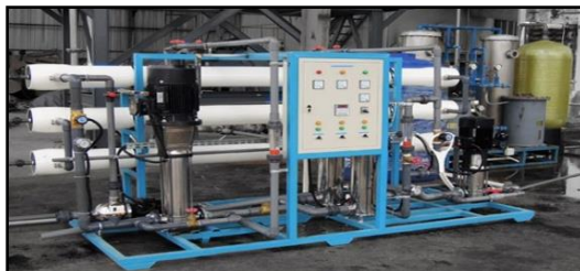
Figure 11. Reverse Osmosis (Source: PT. Nulab Pharmaceutical Indonesia)
