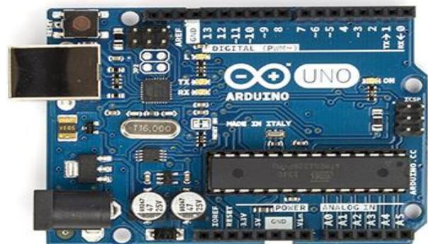
Gambar 4. Arduino Uno rev 3
