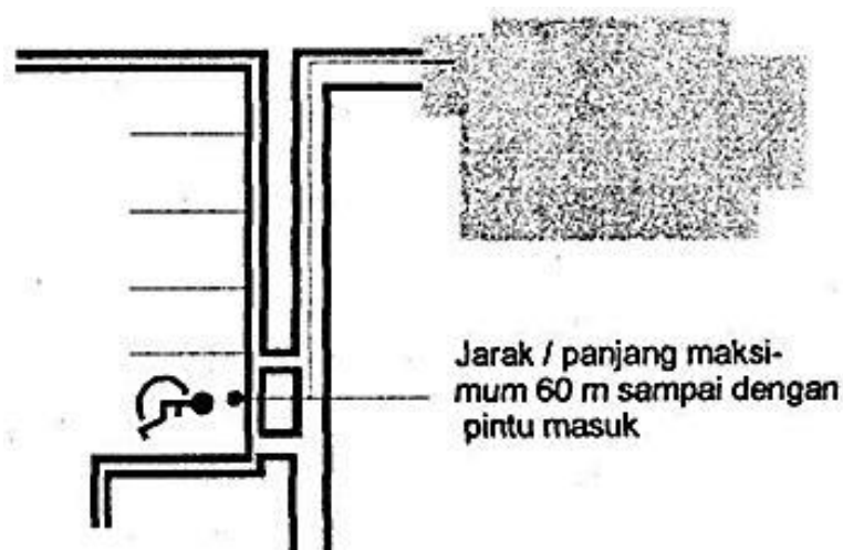
Figure 4. Recommendations for accessible routes for parking areas. Images were taken from https://eprints.uny.ac.id/63842/4/BAB%20II.pdf
