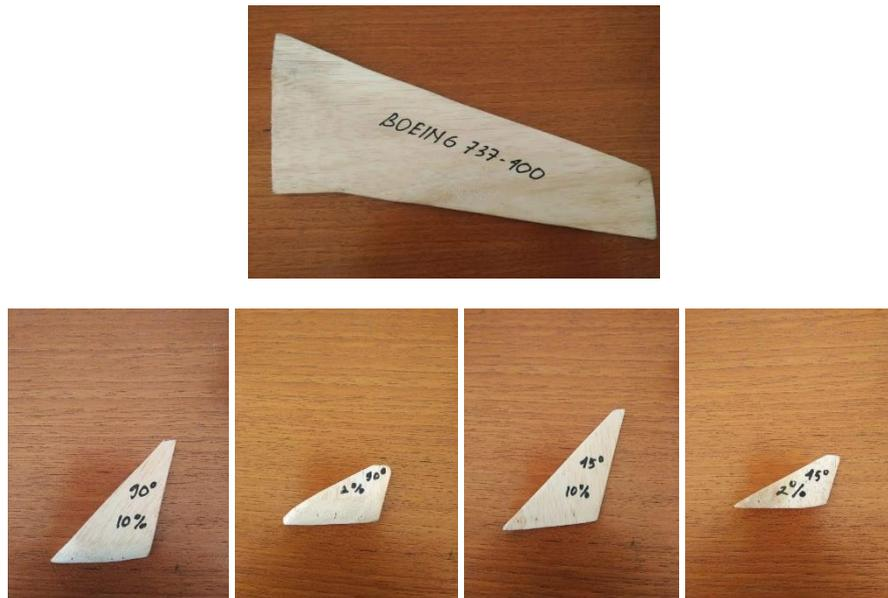
Gambar 5. Model sayap tapered wing dan variasi *blended winglet*
