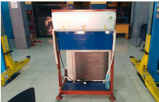
Gambar 5. Alat training unit praktikum A/C split
