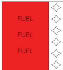
Gambar 3 Sticker identifikasi fuel (Sumber: Aviation Maintenance Technician Handbook, hal. 7-9)
