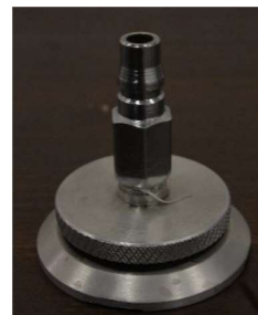
Gambar 6. Vacuum Bagging Port
