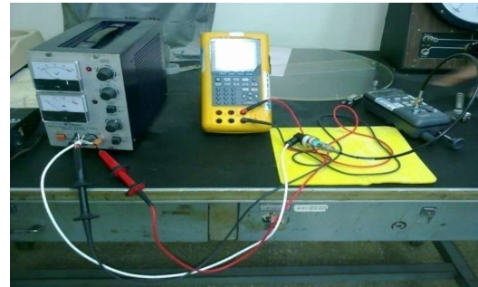
Gambar 4 Proses Pengujian Kalibrasi Transducer
