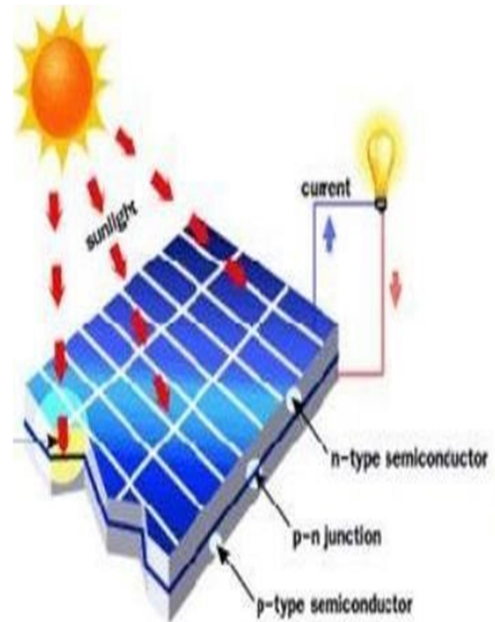
Gambar 1. Ilustrai Prinsip Kerja Solar Cell
