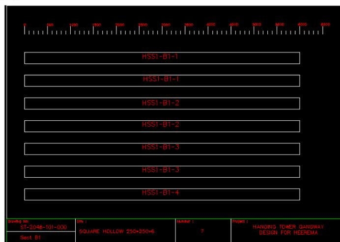
Gambar 3.7 Cutting plan
