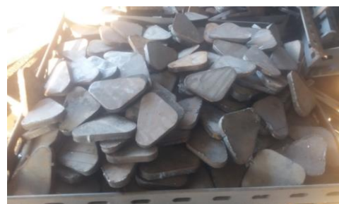
Gambar 3.5 welding pad 75x75x6mm
