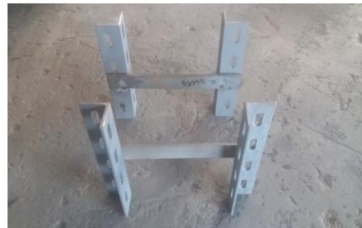
Gambar 3.8 perakitan cable ladder support
