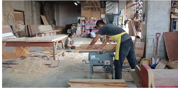
Gambar 1. Proses pengolahan kayu pinus ex pallet (Sumber: Retrieved Juli 30, 2020 from kainafurniture.wordpress.com)
