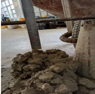
Gambar 4. Slump Test Campuran Beton
