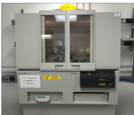
Gambar 1. XRD X'Pert PRO merk PANalytical MPD PW3040/60
