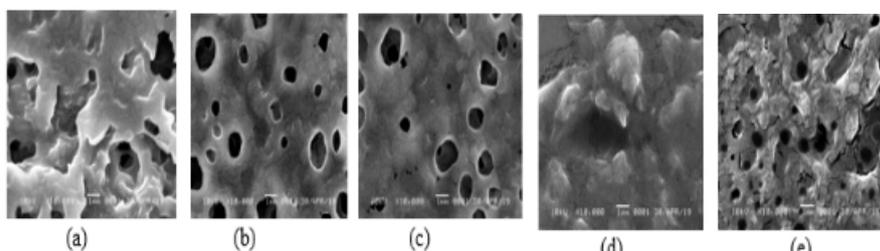
**Fig. 7.** Results of the SEM morphology of NiFe<sub>2</sub>O<sub>4</sub> / PVDF nanocomposites with a magnification of 10,000X, for each composition variation (a) 50%: 50%, (b) 33.3%: 66.6%, (c) 25%: 75% , (d) 75%: 25%, (e) 66.6%: 33.3%
