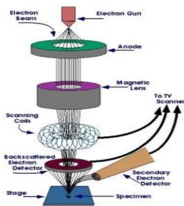
**Fig. 4.** SEM mechanism [14]
