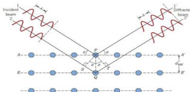
**Fig. 3:** An example of X-ray diffraction on XRD [13].
