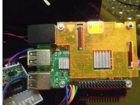
Fig. 6. The Raspberry Pi 3 module installed on the tool
