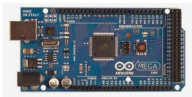
Gambar 2. Arduino Mega 2560
