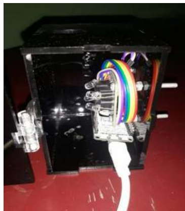
Fig. 6. Position of sensor in acrylic box
