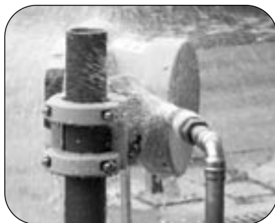
Water Ingress Testing
