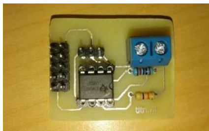
Gambar 12. Hasil rangkaian sensor frekuensi zero crossing detector
