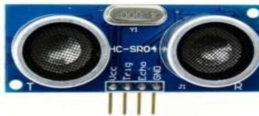
Gambar 4. Sensor Ultrasonik HC SR-04
