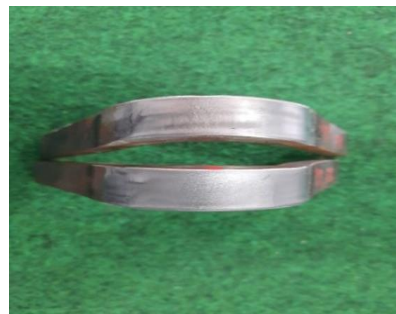
Gambar 7. Hasil pengujian face bending arus 70 A
