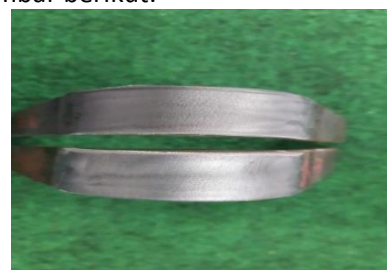
Gambar 8. Hasil pengujian face bending arus 90 A
