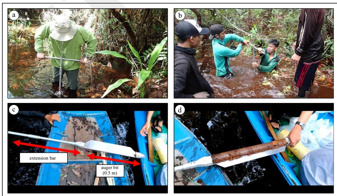
Figure 2. Peat sampling processes. (a) Planting the auger, (b) Rotating the peat sampler, (c) Auger part, (d) Freshly taken peat core.
