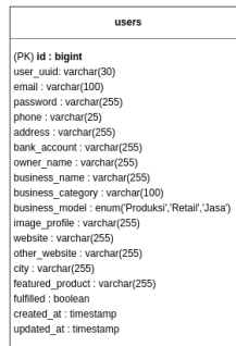
Figure 7. The User service database architecture after refactoring
