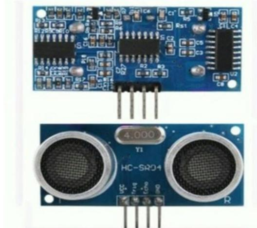
Gambar 2. Sensor ultrasonik HC-SR04
