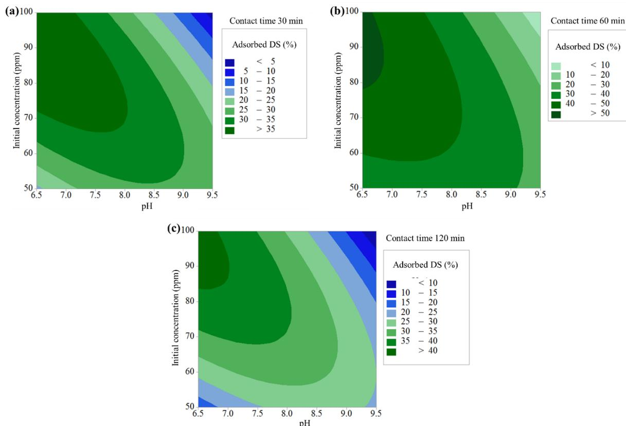
**Figure 5.** Percentage of diclofenac sodium adsorbed on the HDTMA-modified zeolite with a contact time of (a) 30 min, (b) 60 min, and (c) 120 min.
