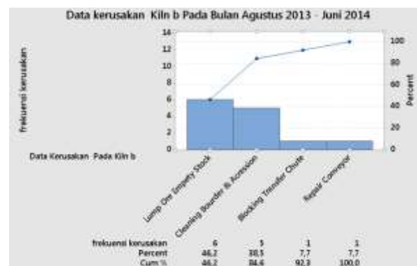
Figure 1. Types of damage and frequency of Rotary Kiln machines b
