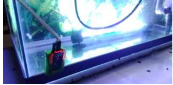
Figure 6. LDR sensor installation
