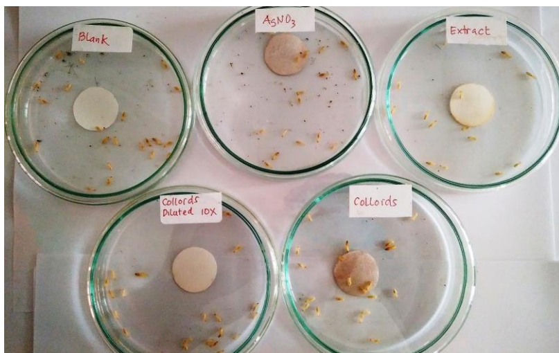
Figure 7. Antitermites test using no-choice method
