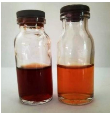
Figure 2. (Left) Reaction mixture under room light irradiation; (Right) reaction mixture in dark condition
