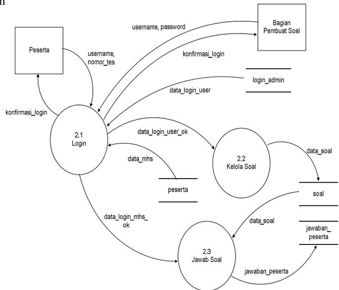
Gambar 5. Diagram Rinci Proses 2.0
