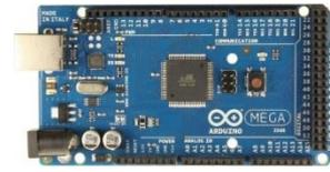
Gambar 2. Arduino Mega
