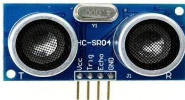
Gambar 6. Sensor Ultrasonik
