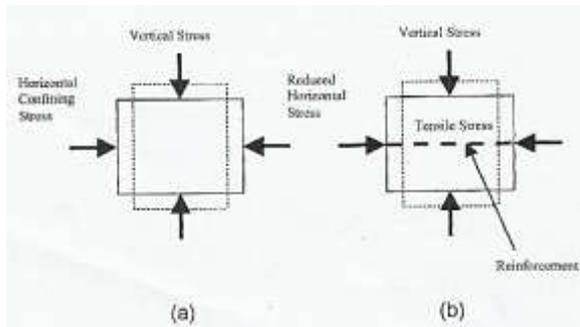
**Gambar 19.** Konsep Dasar *Reinforced Soil System*
