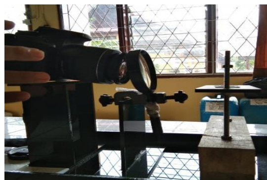
Figure 1. Devices for measuring water contact angles
