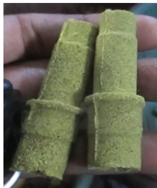
Gambar 1. Material Core berbahan Pasir
