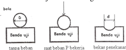
Gambar 4. Prinsip Uji kekerasan brinell (Dieter : 1986)
