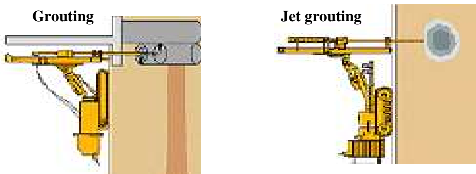
Gb.1. Grouting dan jet grouting
