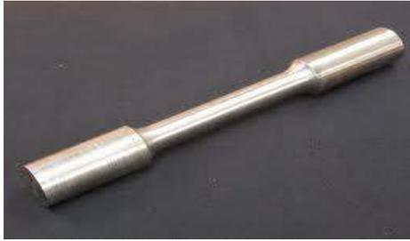
Gambar 3.7 Spesimen uji tarik (standar ASTM E-8)
